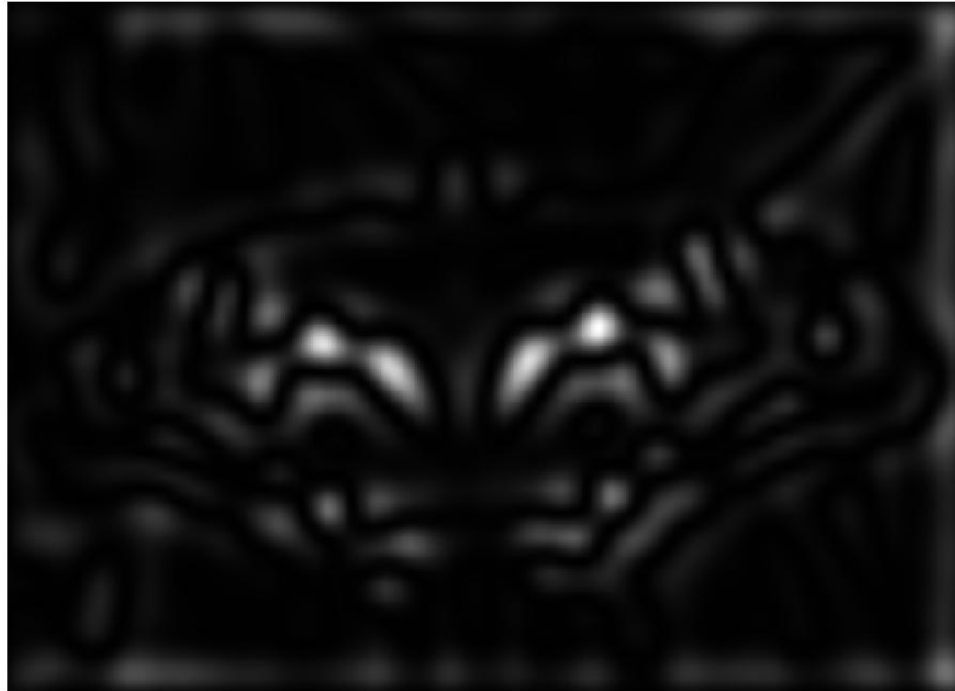
Magnitude of (G(k^9\sigma) - G(k^8\sigma)) | s = 4; \sigma = 1.6 | (third octave shown at the input resolution for convenience)
