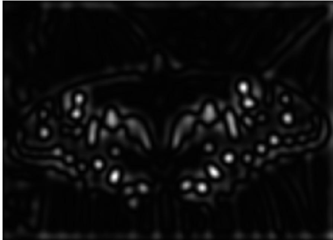
Magnitude of (G(k^7\sigma) - G(k^6\sigma)) | s = 4; \sigma = 1.6 | (second octave shown at the input resolution for convenience)
