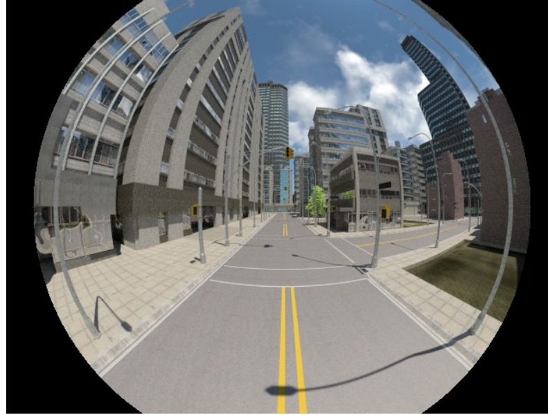
Fisheye (highest resolution is achieved around the optical axis)
