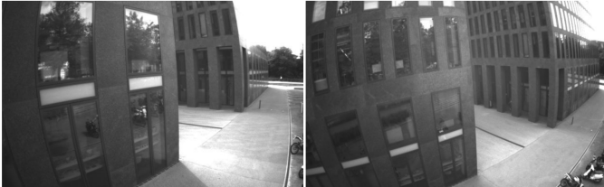
Fig. 9: Images of the same part of the building taken in two consecutive laps. Neither SVO-Loop Closure nor ORB-SLAM3 can close a loop based on visual descriptor matching. Contrary, our map registration is performed successfully in this situation.
