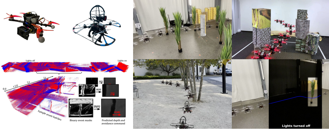
Figure 5: (top left) The two quadrotor platforms used for indoor and outdoor experiments with different event cameras. The Falcon250 [30] additionally has a VOXL board [31] for state estimation. (lower left) An event-volume (10% true density) produced by the continuous event stream from the in-the-dark trial, with select event batches, corresponding BEMs, and network predictions shown. Note the high density of negative (blue) events and positive (red) events when the lights turn off and on, respectively. (right) A variety of real experiments in indoor and outdoor conditions. Our event camera-equipped quadrotor can avoid obstacles in the dark, where traditional cameras would fail.
