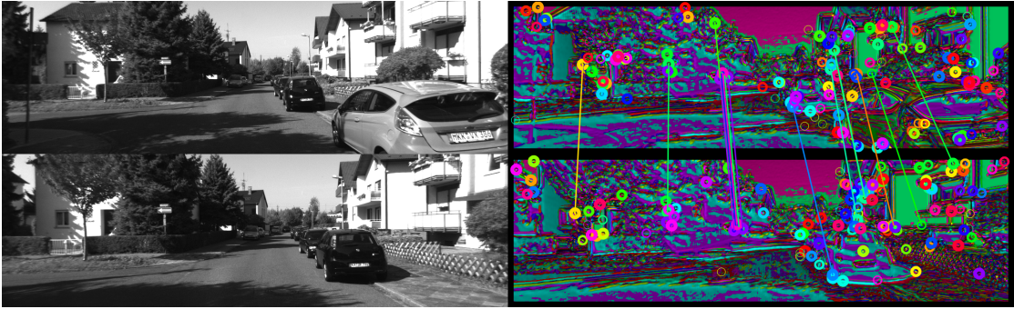
Figure 2.12 – Input and output of our implicitly matched feature detection network for the same image pair as in Figure 2.9. This is the output with 128 output channels, circles indicate points selected by the channels, hue stands for channel identity. Additionally, the hue of each pixel indicates which channel has the highest response at that pixel. Brightness indicates the strength of the response. Lines connect inlier matches that can be used for relative pose estimation between the two images.
