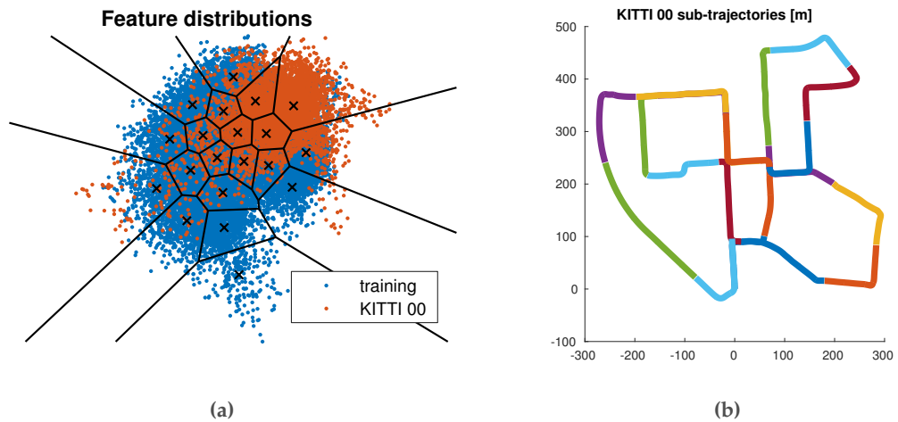
Figure 2.3 – (a) The clustering of the image descriptor space, illustrated on a projection of the space onto two dimensions. Note the difference between the training distribution and the distribution when evaluating on KITTII 00. This results in an uneven load balancing. (b) We simulate n agents by subdividing a single-agent dataset, here KITTII 00, into n parts. Simulated place recognition between agents occurs on portions of the trajectory that are observed multiple times in the single-agent recording.
