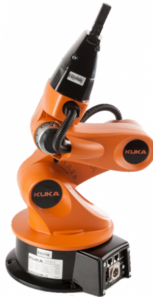
Figure 2.2: The 5 DoF arm of the KUKA youBot
