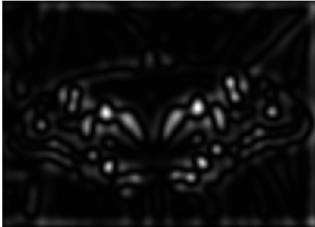
Magnitude of (G(k^8\sigma) - G(k^7\sigma)) | s = 4; \sigma = 1.6 | (second octave shown at the input resolution for convenience)
