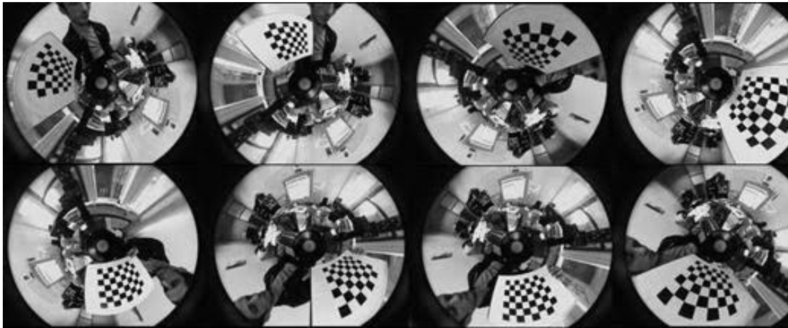
Example calibration images of a catadioptric camera
