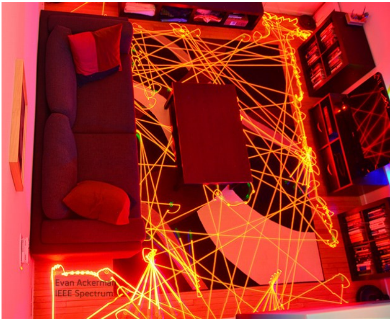
The Roomba 880 navigates by zigzagging randomly across the room. Average cleaning time: 20 minutes
