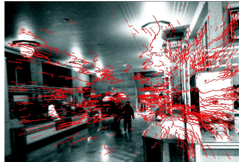
Features tracked over multiple recent frames overlaid on the last frame
