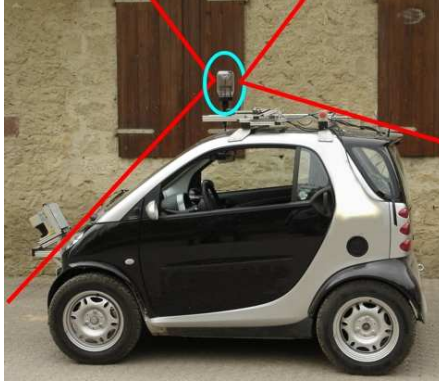
Figure 7.1: The vehicle used in our experiments equipped with the omnidirectional camera (blue circle). The vertical field of view is indicated by the red lines.
