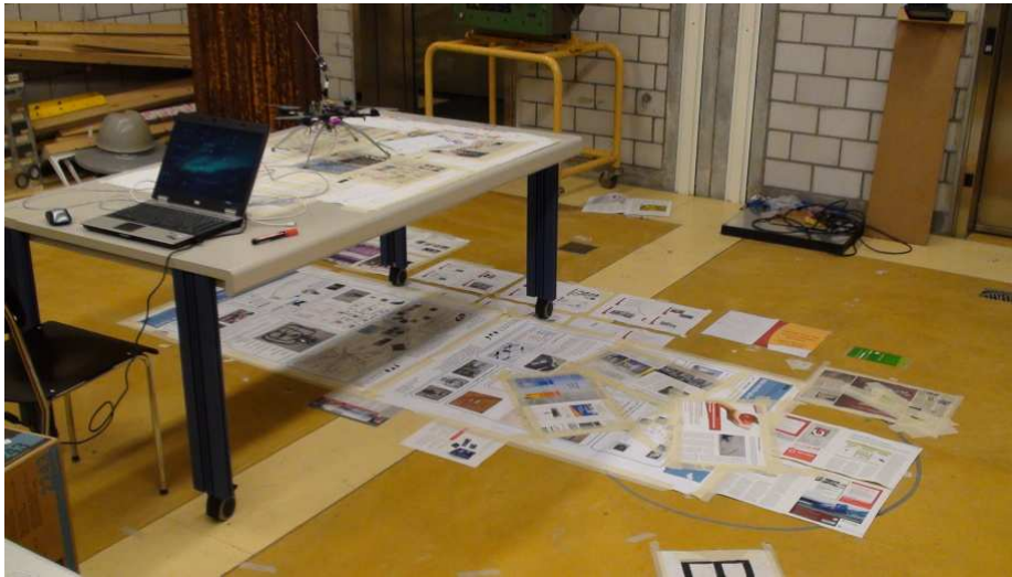
Fig. 11 Test arena for our MAV. As test sequence we started on the table and flew to the right. As soon as the textured 3D mesh map indicated us that it is safe to descend (i.e. that we do not hit the table) we approached the floor to get a higher resolution of the floor for the map. After, we ascended and returned to the starting position on the table always using the information of the intuitive 3D map.
