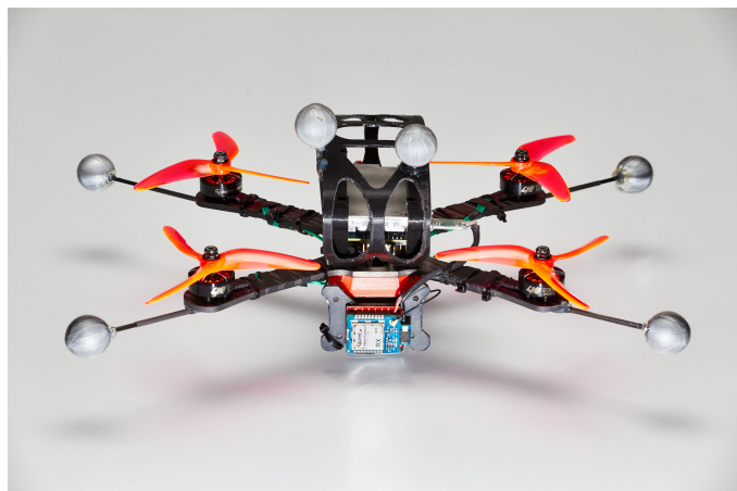
Fig. 12: The quadrotor platform that is used for real-world experiments. The achievable thrust-to-weight ratio is 4. The platform is equipped with a Laird module for real-time wireless communication, off-the-shelf components, and reflecting markers for the VICON localization system.
