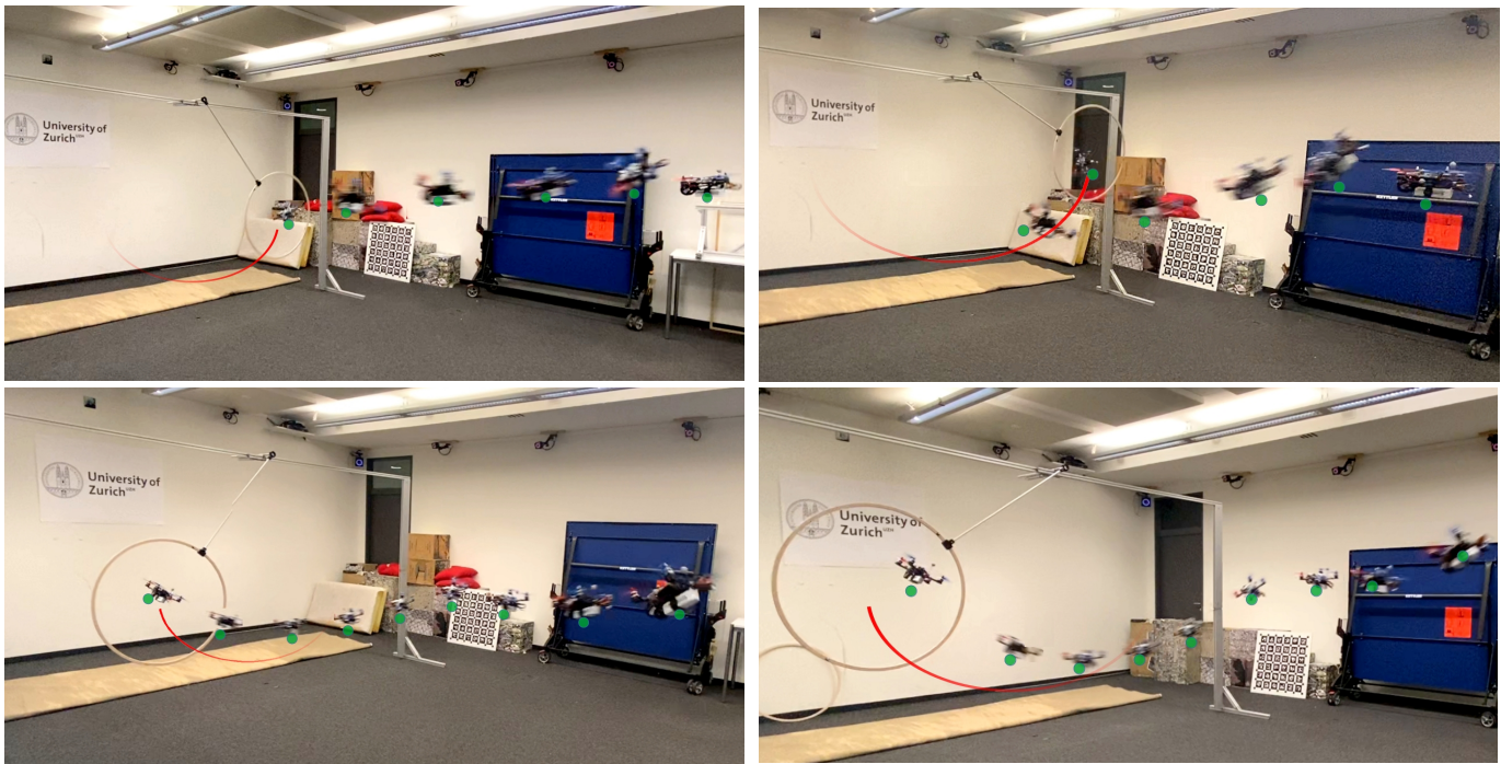
Fig. 12: Controlling a quadrotor to fly through a dynamic gate using High-MPC under random initializations.
