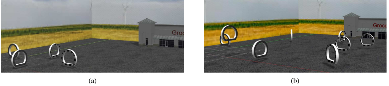
Fig. 4: Illustration of the simulated tracks. The small track (a) consists of 4 gates and spans a total length of 43 meters. The large track (b) consists of 8 gates placed at different heights and spans a total length of 116 meters.
