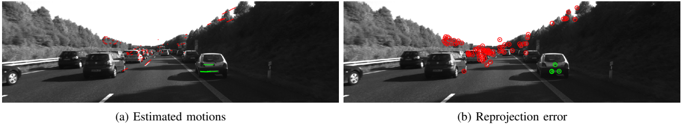
Fig. 8: Traffic jam sequence (sequence car_20_02 ): due to traffic jam, all cars but one are almost still and get classified as static part of the scene (red).
