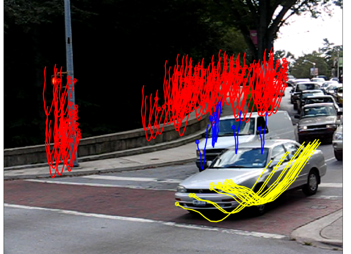
Fig. 1: Estimated motions: ego-motion in red and eoru-motion in yellow and blue .
