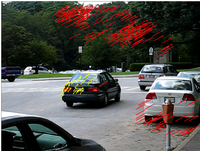
(a) Estimated motions: ego-motion in red and eoru-motion in yellow.
