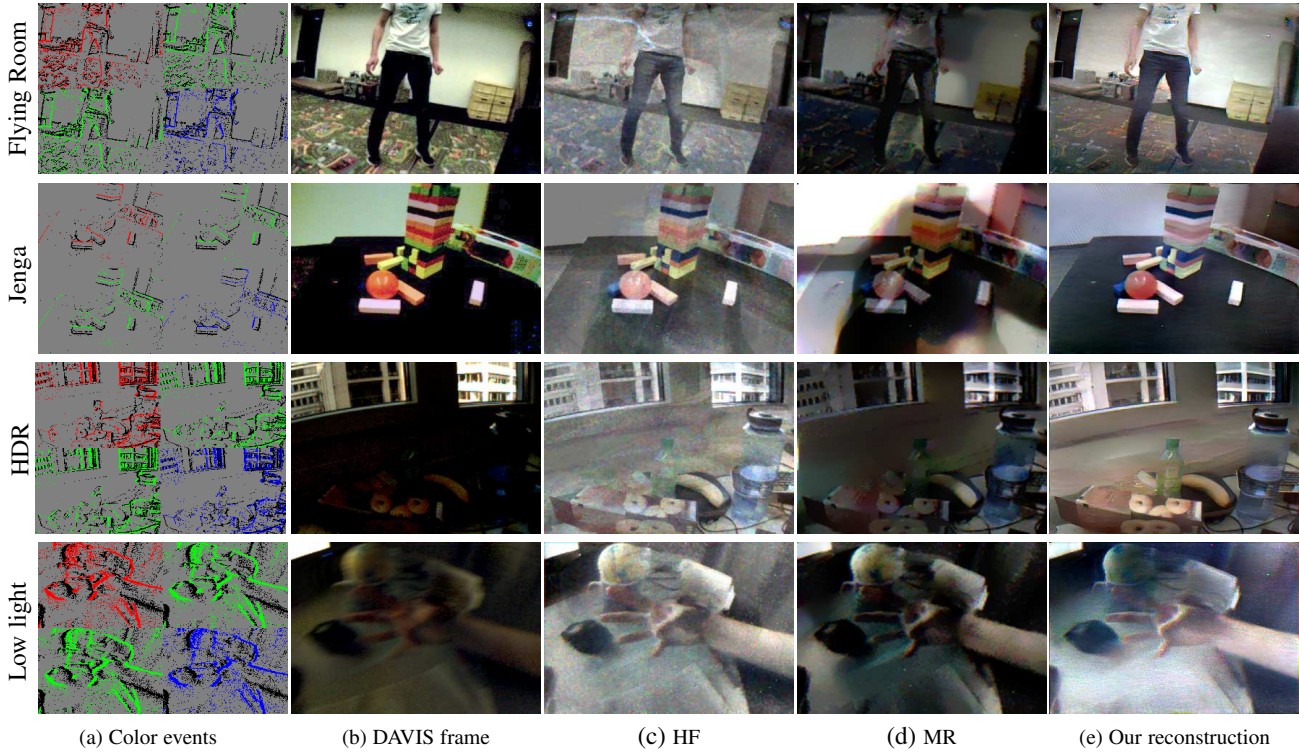
Fig. 11. Color reconstruction results from color events (a) using datasets from [45], comparing a conventional frame (b) with multiple reconstructions from events only: HF (c), MR (d), and ours (e). For visualization, the color events (a) are split into each color channel. Positive (ON) events are colored by the corresponding filter color, and negative (OFF) events are black.
