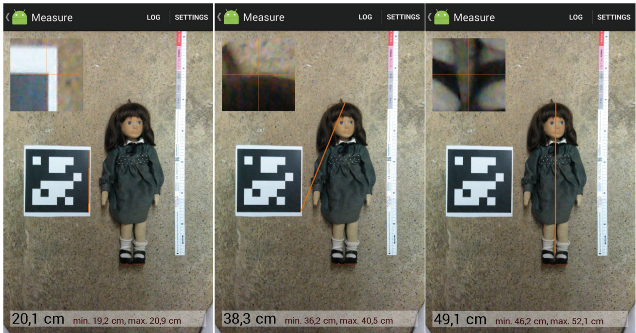
Fig. 1 Example pictures of the “Optisizer” App. At first, a picture is taken with tag and child. The tag is recognized by the app and the body length has to be manually tagged at the upper limit ( middle picture )
