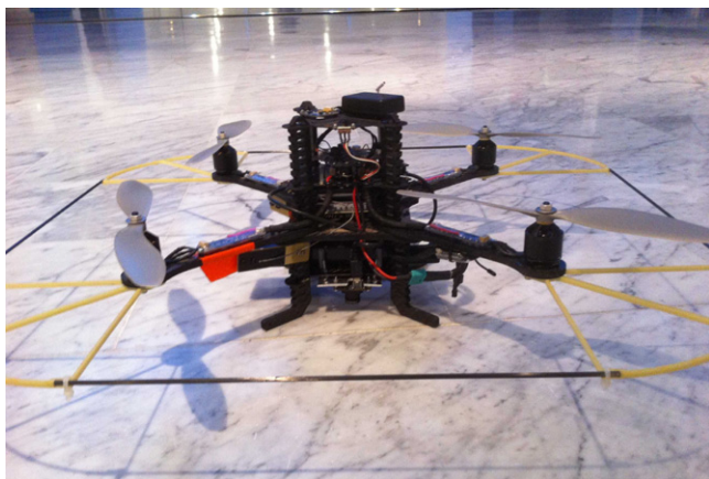
Fig. 31. AscTec Pelican quadcopter [55] equipped with a monocular camera.
