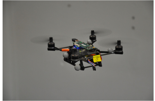
Fig. 23. Our nano quadrotor from KMeI Robotics: a 150 g and 18 cm sized platform equipped with an integrated Gumstix Overo board and MatrixVision VGA camera.
