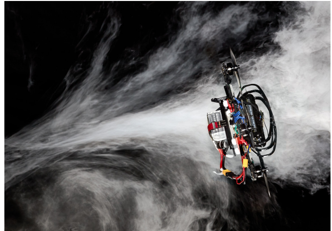
Fig. 1. The proposed algorithm is able to adapt on-the-fly when encountering unknown disturbances. In the figure we show a quadrotor platform flying at speeds of more than 60 km/h. Thanks to our online replanning method, the drone can adapt to wind disturbances of up to 68 km/h while flying as fast as possible.
