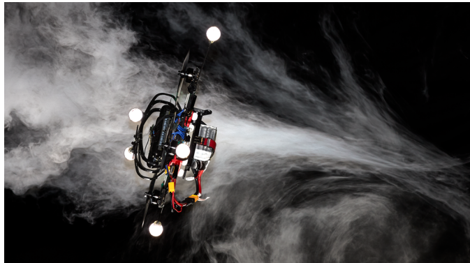
Fig. 1: Our quadrotor platform reaches its physical limits at a pitch angle of 80 degrees while performing a lemniscate trajectory in our experiments. Throughout the trajectory, the platform reaches speeds of up to 14\text{m s}^{-1} and accelerations beyond 4g.
