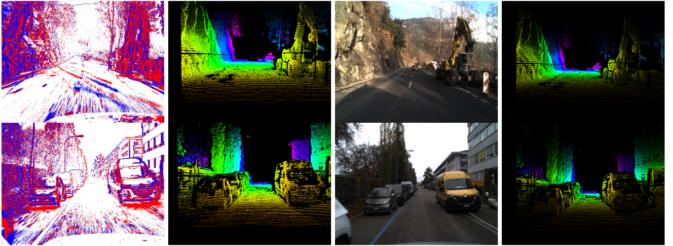
Fig. 7: Examples of recorded event and image data with corresponding disparity groundtruth. From left to right: events with the corresponding disparity and image with corresponding disparity. The disparity image is colored to provide a sense of depth.
