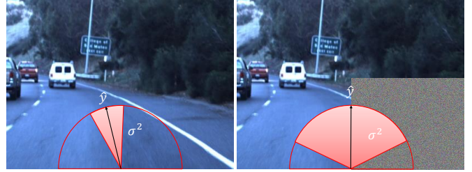
Fig. 1. A neural network trained for steering angle prediction can be fully functional on a clean image (left) but generate unreliable predictions when processing a corrupted input (right). In this work, we propose a general framework to associate each network prediction with an uncertainty (illustrated above in red) that allows to detect such failure cases automatically.
