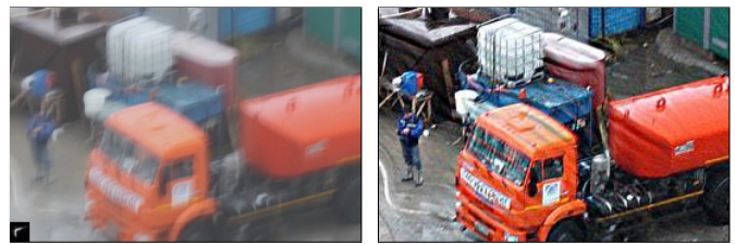
(a) Blurred image. The blur kernel (PSF) is shown in a corner. (b) Restored image (blur corrected, but still with artifacts).
