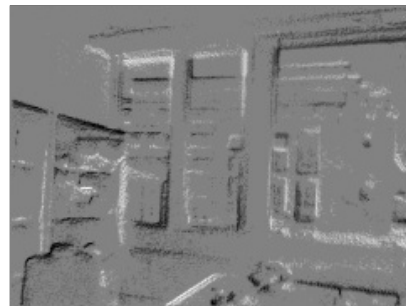
(b) Image of rotated events, i.e., after motion compensation. I(\mathbf{x}; \omega) is given by (4) with the optimal \omega . Observe how sharp the edges are everywhere in the image, even far away from the center of rotation.
