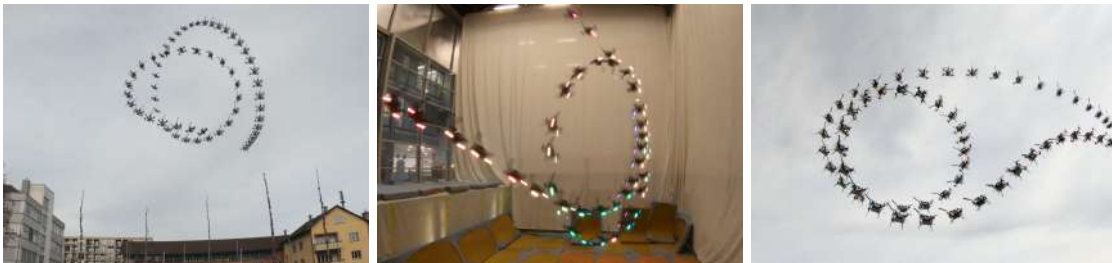
Figure 2.4 – A quadrotor performs a Barrel Roll (left), a Power Loop (middle), and a Matty Flip (right). We safely train acrobatic controllers in simulation and deploy them with no fine-tuning ( zero-shot transfer ) on physical quadrotors. The approach uses only onboard sensing and computation. No external motion tracking was used.
