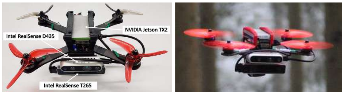
Figure S1 – Illustration of our experimental platform. The main computational unit is an NVIDIA Jetson TX2, whose GPU is used for neural network inference and CPU for the control stack. Sensing is performed by an Intel Realsense T265 for state estimation and an Intel Realsense D435 for depth estimation.
