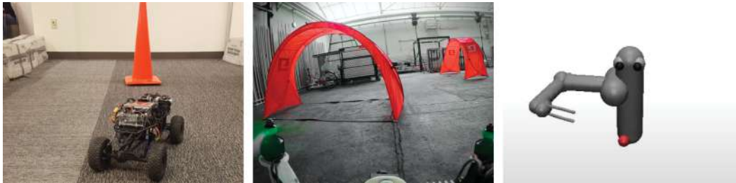
Figure 1.16 – Estimating uncertainty is of paramount importance to integrate learning-based methods into robotics systems. Kahn et al. [133] used model-uncertainty to speed-up the learning process for an autonomous car (left). Kaufmann et al. [137] estimated the uncertainty of gate detection to enable bayesian decision making during drone racing (center). Chua et al. [41] accounted for model errors during model-based reinforcement learning by leveraging their uncertainty (left).
