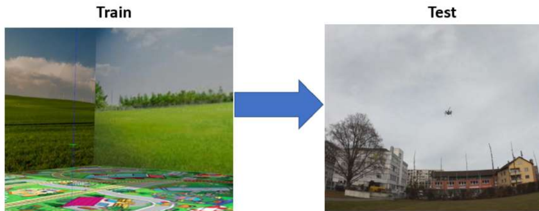
Figure 1.5 – Learning the complex mapping between noisy sensor observations and actions generally requires large and diverse training datasets. Collecting these datasets in the real world is a tedious and expensive procedure, that also raises fundamental questions on how to sufficiently cover the state space to enable closed-loop performance. To address this problem, I propose to train sensorimotor policies entirely in simulation and then transfer the acquired knowledge to a physical platform via domain-invariant abstraction.
