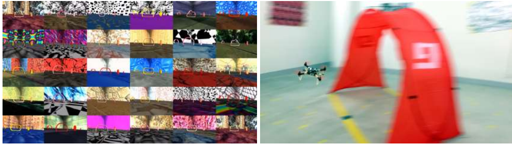
Figure C.1 – The perception block of our system, represented by a convolutional neural network (CNN), is trained only with non-photorealistic simulation data. Due to the abundance of such data, generated with domain randomization, the trained CNN can be deployed on a physical quadrotor without any finetuning.
