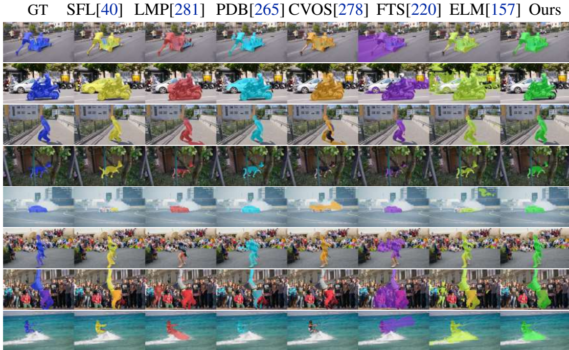
Figure B.4 – Qualitative Results: We qualitatively compare the performance of our approach with several state-of-the-art baselines as well as the Ground-Truth (GT) mask. Our prediction is robust to background clutter, large depth discontinuities and occlusions. The last row shows a typical failure case of our method, i.e. objects which are moved by the primary objects are detected as foreground (water is moved by the surfer in this case).
