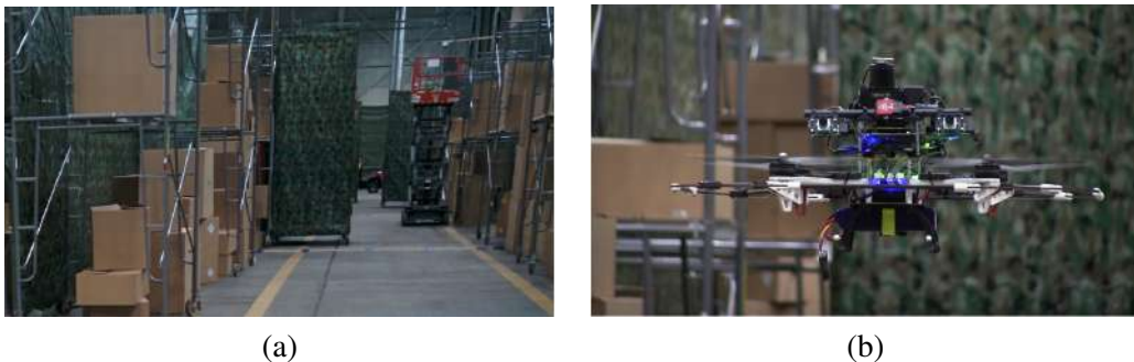
Figure 1.9 – The system proposed by Mohta et al. can navigate previously unknown environments with only on-board sensing and computation (a). However, it relies on a bulky computational and sensing unit (b), which limits the agility and speed of the system.
