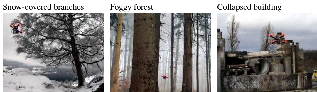
Figure 2.5 – Samples of man-made and natural environments where our sensorimotor policy has been deployed. All environments are previously unknown. The navigation policy was trained entirely in simulation and uses only onboard sensing and computation.
