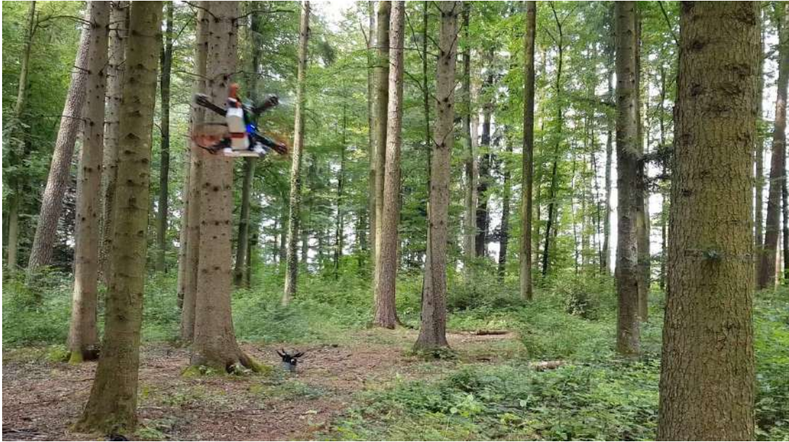
Figure 1.1 – A tightly-coupled perception-action loop, powered by the combination of traditional model-based robotics and state-of-the-art machine learning tools, enables autonomous high-speed operation in unstructured environments. The quadrotor is required to reach a waypoint 50 meters in front of it given by a user. The environment is not known in advance, and the robot has only access to on-board sensing and computation (no GPS or external tracking systems are used).
