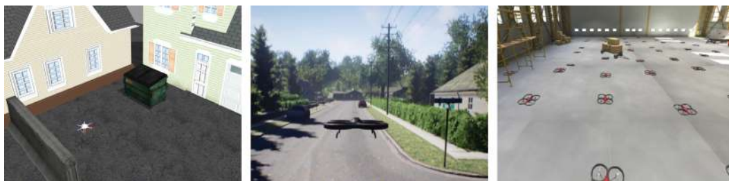
Figure 1.13 – Several quadrotor simulators are available to develop, train, and test navigation algorithms. While some offer very accurate dynamics (left) [78], others have highly photo-realistic rendering (center) [257]. I have contributed to build Flightmare (right) [266], a simulator which offers both and is specifically tailored to machine learning applications.
