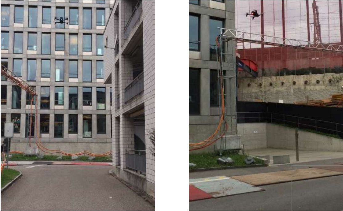
Figure A.7 – High altitude Outdoor 1: In order to test the ability of DroNet to generalize at high altitude, we made the drone fly at 5 m altitude in the testing environment Outdoor 1 . Table A.2 indicates that our policy is able to cope with the large difference between the viewpoint of a camera mounted on a car (1.5 m) and the one of the UAV.
