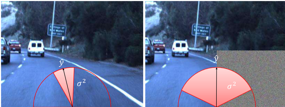
Figure 2.7 – A neural network trained for steering angle prediction can be fully functional on a clean image (left) but generate unreliable predictions when processing a corrupted input (right). In this chapter, I propose a general framework to associate each network prediction with an uncertainty (illustrated above in red) that allows the detection of such failure cases automatically.
