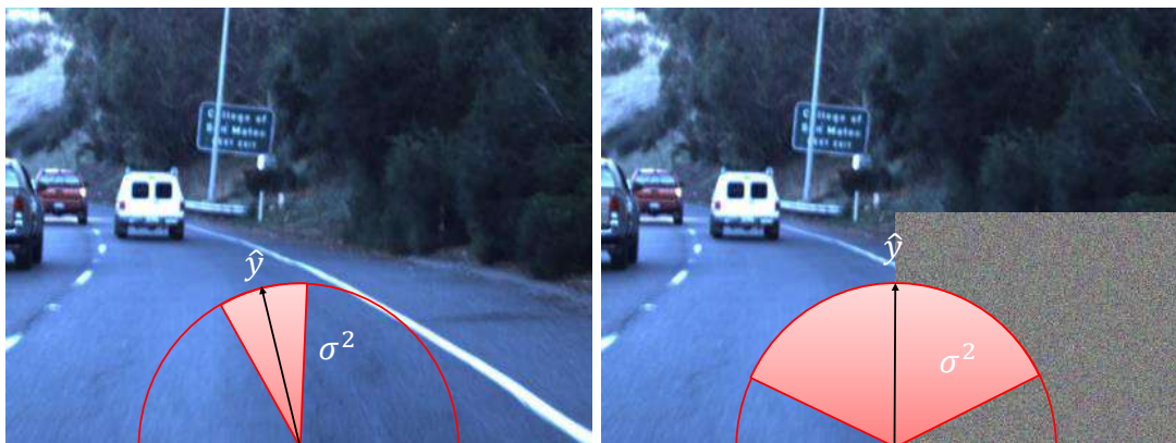
Figure D.1 – A neural network trained for steering angle prediction can be fully functional on a clean image (left) but generate unreliable predictions when processing a corrupted input (right). In this work, we propose a general framework to associate each network prediction with an uncertainty (illustrated above in red) that allows to detect such failure cases automatically.
