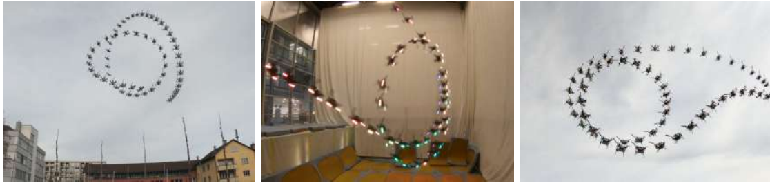
Figure F.1 – A quadrotor performs a Barrel Roll (left), a Power Loop (middle), and a Matty Flip (right). We safely train acrobatic controllers in simulation and deploy them with no fine-tuning ( zero-shot transfer ) on physical quadrotors. The approach uses only onboard sensing and computation. No external motion tracking was used.
