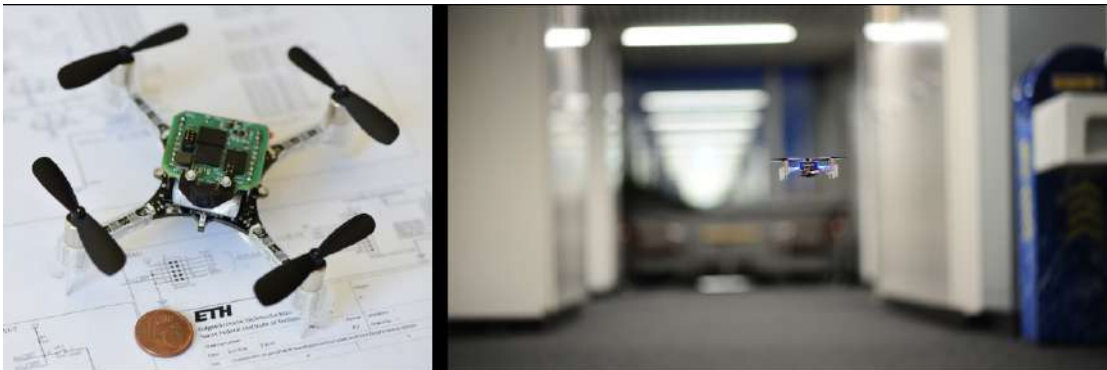
Figure 2.2 – PULP-DroNet: a deep learning-powered visual navigation engine that enables autonomous navigation of a pocket-size quadrotor in a previously unseen environment.
