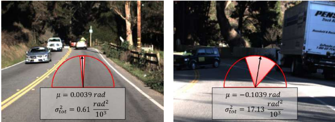
Figure D.3 – On well illuminated frames where the car is driving straight, a network trained to predict steering angles is very certain about its output (left). In contrast, for poorly illuminated, ambiguous frames, the network is highly uncertain about its predictions (right).
