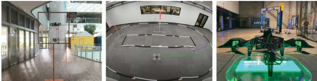
Figure 1.14 – The classic approach to autonomous drone racing is to detect the next gate and steer the drone towards it (left) [131]. To account for the cases when no gate is visible, it is possible to combine state estimation and gate detection through Kalman filtering (right) [71]. Multi-agent autonomous drone racing also raises interesting game-theoretical problems (center) [267].
