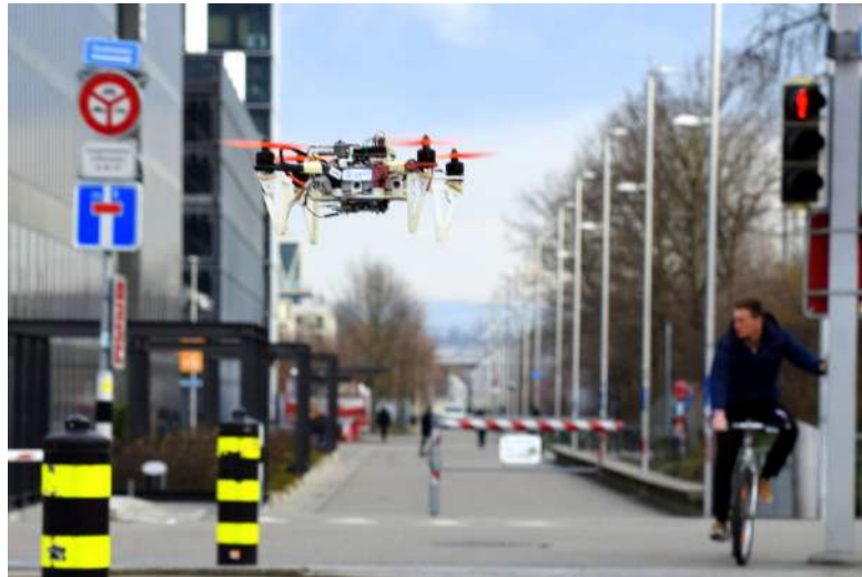
Figure A.1 – DroNet is a convolutional neural network, whose purpose is to reliably drive an autonomous drone through the streets of a city. Trained with data collected by cars and bicycles, our system learns from them to follow basic traffic rules, e.g. do not go off the road, and to safely avoid other pedestrians or obstacles. Surprisingly, the policy learned by DroNet is highly generalizable, and even allows to fly a drone in indoor corridors and parking lots.
