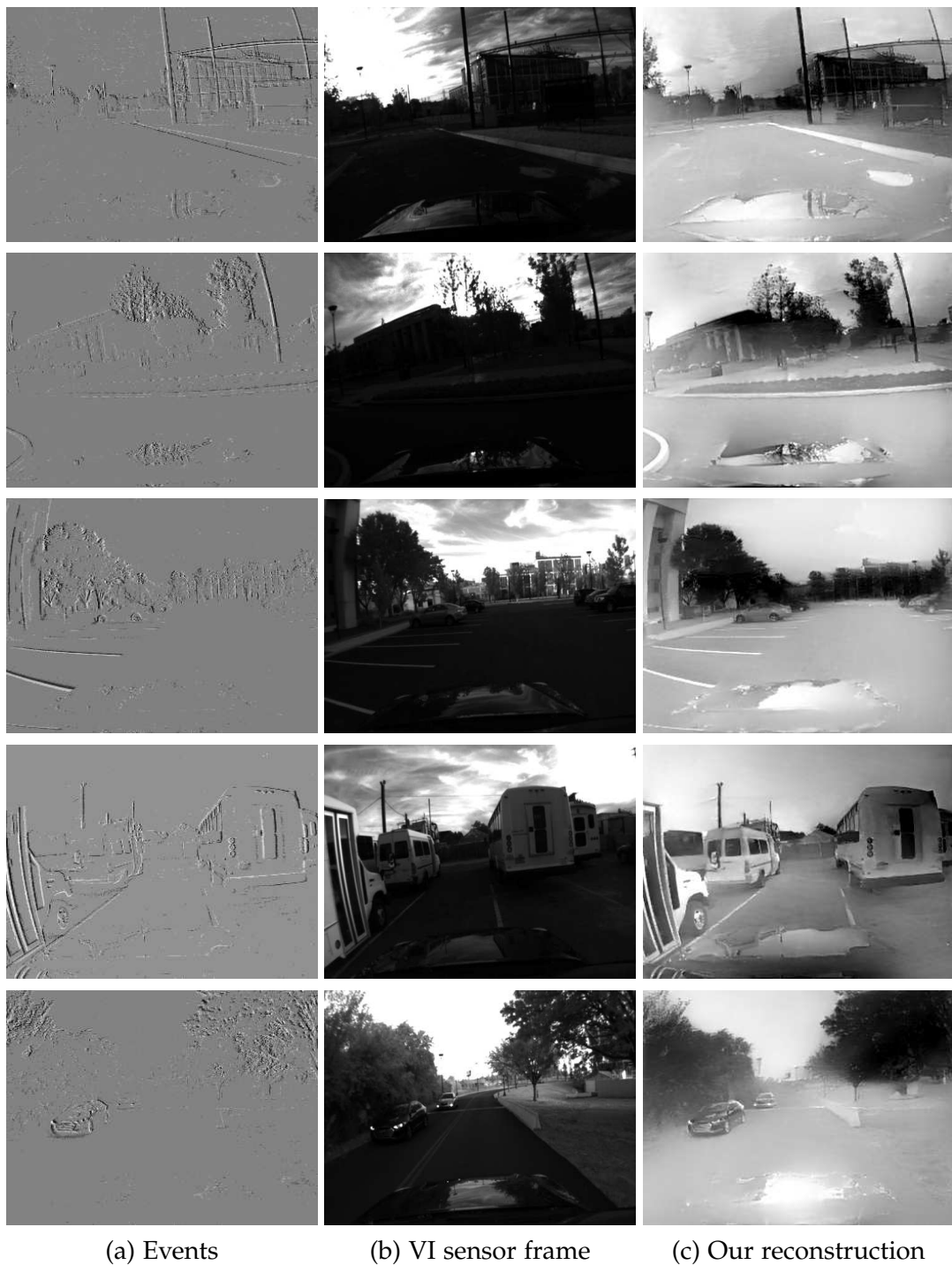
Figure F.21 – Example HDR reconstructions on the MVSEC automotive dataset [212]. The standard frames were recorded with a high-quality VI sensor with auto-exposure activated. Because the camera is facing directly the sun, the standard frames (b) are either under- or over-exposed since the limited dynamic range of the standard sensor cannot cope with the high dynamic range of the scene. By contrast, the events (a) capture the whole dynamic range of the scene, which our method successfully reconstructs to high dynamic range images (c), allow to discover details that were not visible in the standard frames.
