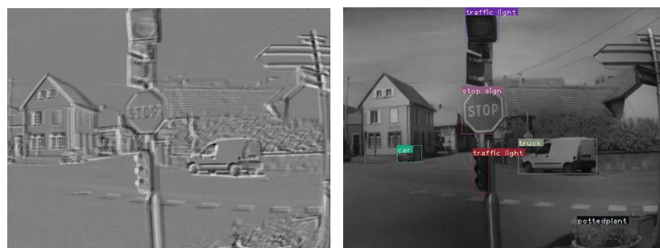
(b) Object detection from events. Left: events. Right: reconstruction and predicted labels [158].
