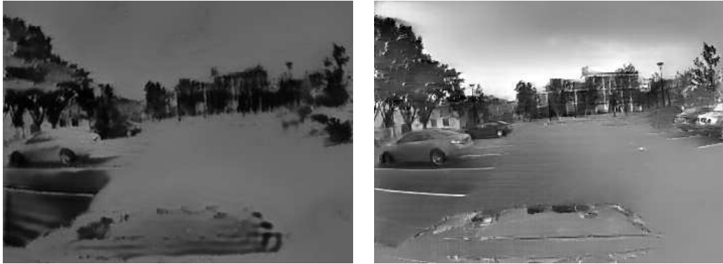
Figure F.17 – Reconstruction from (i) a network trained only on real event data from the DAVIS240C sensor (left), and (ii) a network trained only on simulated event data (right). This sequence is from the MVSEC dataset, and was recorded with a mDAVIS346 sensor.
