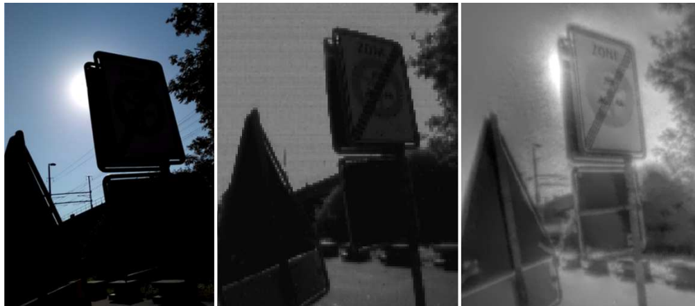
Figure C.12 – Outdoor sequence, pointing at the sun. Left: View from a standard camera, showing severe under-exposure on the foreground. Middle: Frame from the DAVIS, showing severe under- and over-exposed areas. Right: HDR image reconstructed using the output of EVO.
