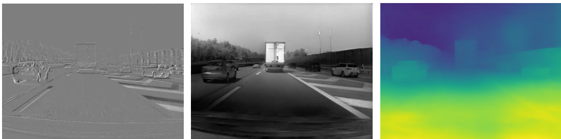
(a) Monocular depth from events. Left to right: events, reconstruction, predicted depth [97].
