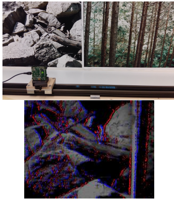
(a) Constant illumination setup. Events on a frame.
