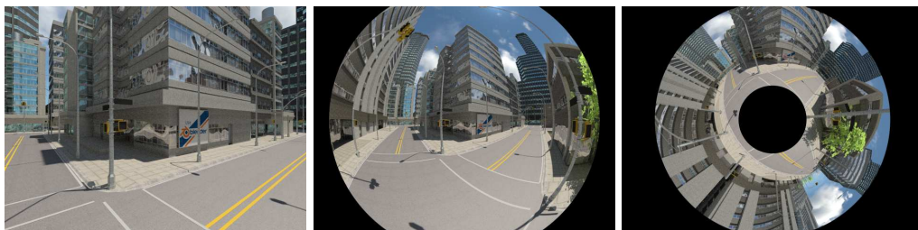
Figure 2.12 – Images from our MultiFOV synthetic datasets [207]. From left to right: simulated pinhole, fisheye and catadioptric lenses.
