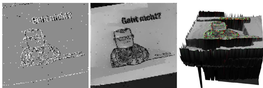
Figure 1.19 – Intensity reconstruction using manifold regularization [125]. From left to right: raw events, reconstruction result, and visualization of the surface of active events , which records the time of the last event at each pixel.
