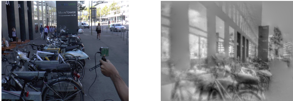
Figure C.11 – Impressions of the outdoor dataset. Left: image from the DAVIS. Right: reconstructed image using the output of EVO. Observe that the reconstructed image is not over- or under-exposed.
