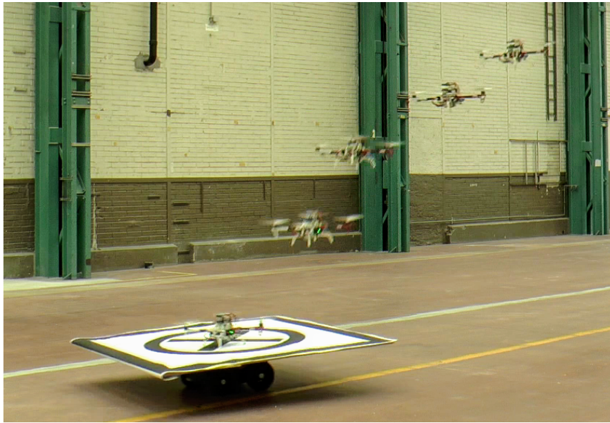
Figure F.1: Our quadrotor during the landing on a moving platform.
