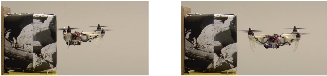
Figure E.7: Inspection of a surface using the T configuration (left) and the X configuration (right).
