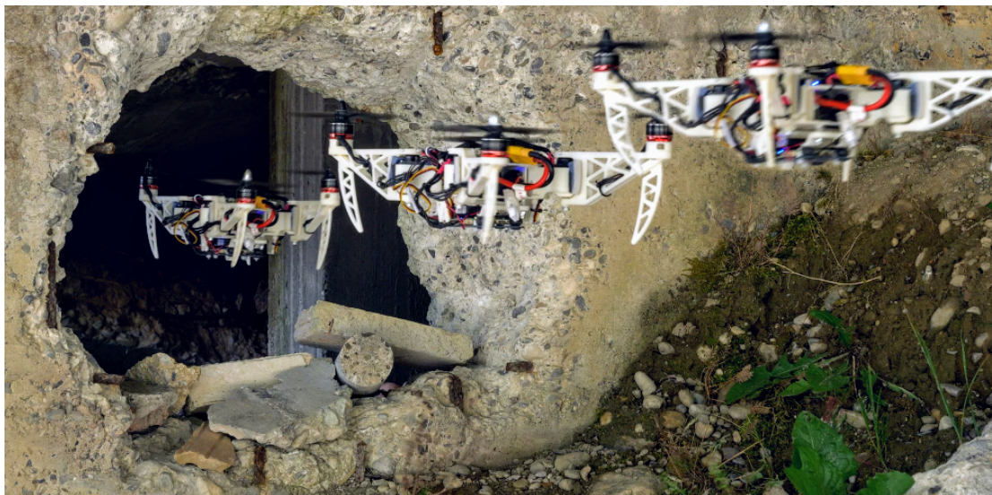
(d) Traverse of a narrow gap to enter a collapsed building.
