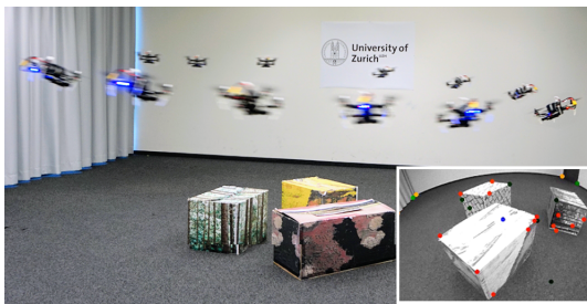
(a) The quadrotor flying along a circle trajectory, while tracking the boxes in the center thanks to perception term in the cost function.
