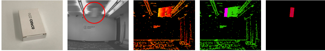
(b) A small-sized marker (width 6 cm, height 9.5 cm, thickness 2.5 cm).
