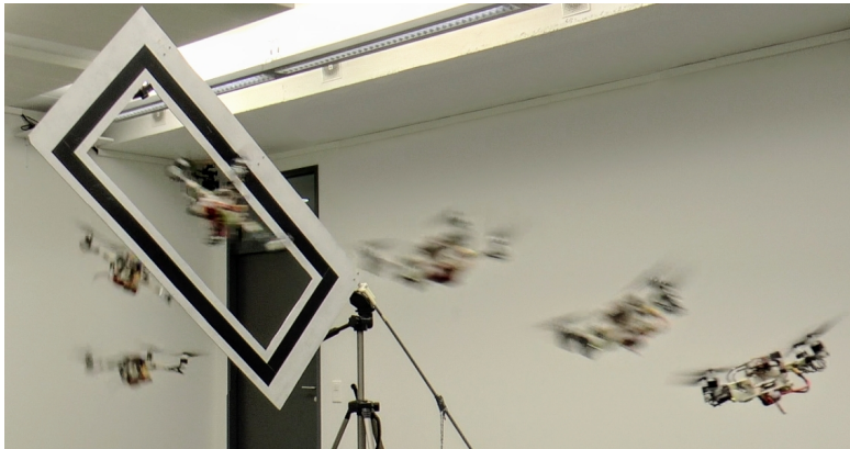
(a) The quadrotor passing through the gap.
