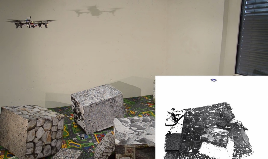
Figure A.7: Our flying arena equipped with an OptiTrack motion-capture system (for ground-truth recording), carpets and boxes for 3D structure.
