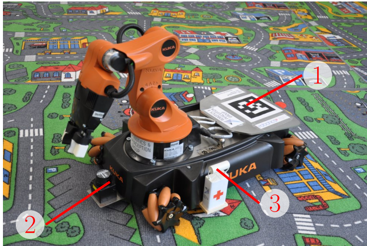
Figure D.3: KUKA youBot equipped with an AprilTag (1), a laser scanner (2), and a first-aid kit (3).
