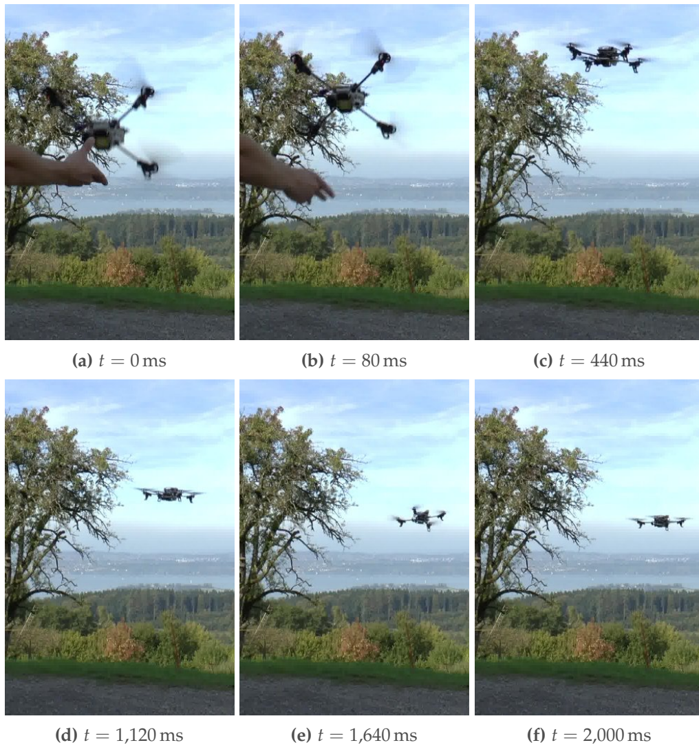
Figure B.1: Autonomous recovery after throwing the quadrotor by hand: (a) the quadrotor detects free fall and (b) starts to control its attitude to be horizontal. Once it is horizontal, (c) it first controls its vertical velocity and then, (d) its vertical position. The quadrotor uses its horizontal motion to initialize its visual-inertial state estimation and uses it (e) to first break its horizontal velocity and then (f) lock to the current position.
