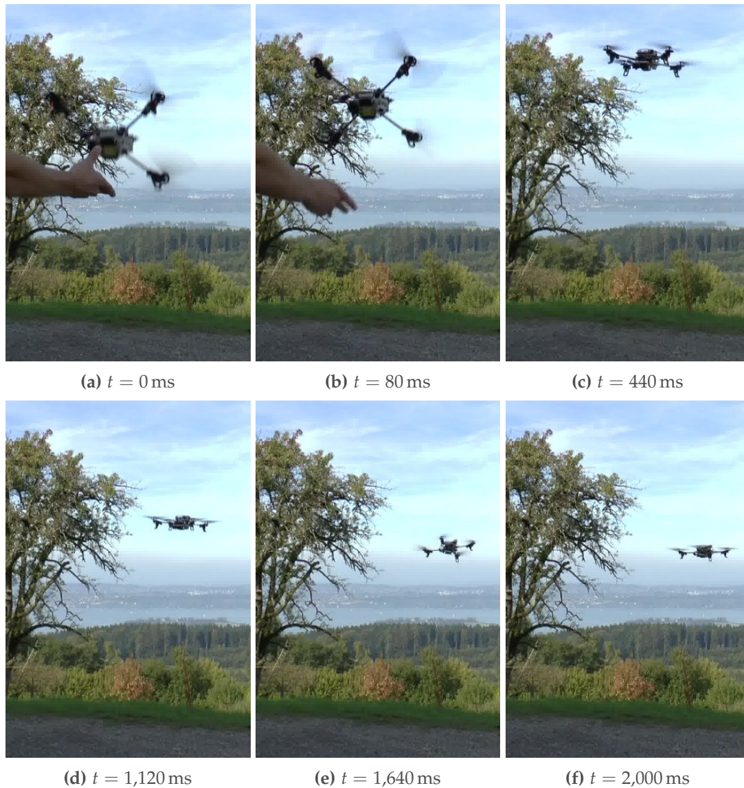
Figure 2.2: Autonomous recovery after throwing the quadrotor by hand: (a) the quadrotor detects free fall and (b) starts to control its attitude to be horizontal. Once it is horizontal, (c) it first controls its vertical velocity and then, (d) its vertical position. The quadrotor uses its horizontal motion to initialize its visual-inertial state estimation and uses it (e) to first break its horizontal velocity and then (f) lock to the current position.
