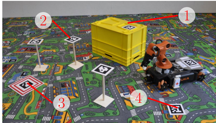
Figure D.4: Mock-up disaster site elements: fixed obstacle (1), movable obstacle (2), goal (3), and origin tag (4).
