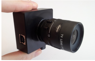
(a) The Dynamic Vision Sensor (DVS).
