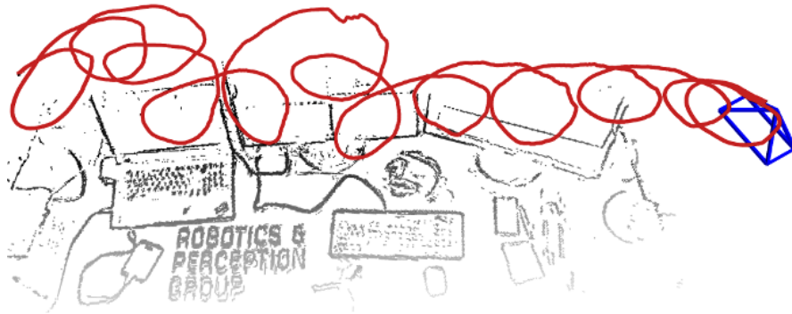
Figure 1.13: EVO [124]: geometric approach to 6-DOF semi-dense parallel tracking and mapping in real time on a CPU.
