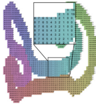
Figure J.3: Mapping from each pixel location to the nearest track vertex speeds up lookup of the nearest track vertex (number at each pixel location).
