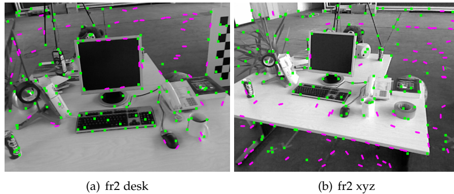
Figure B.13 – Impressions from the TUM RGB-D benchmark dataset Sturm et al. [2012] with tracked corners in green and edgelets in magenta.
