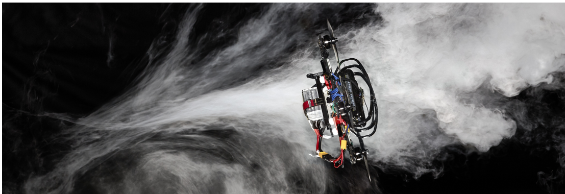
Figure 2.4: A quadrotor in a high-acceleration flight maneuver through smoke to visualize the air flow around the vehicle. Real-world flight data can be used to estimate and model the residual aerodynamic forces not explained by the rigid-body quadrotor dynamics.
