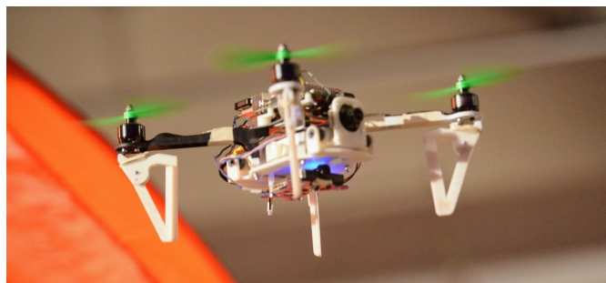
Figure F.4: Our platform, equipped with an Intel UpBoard and a Qualcomm Snapdragon Flight.
