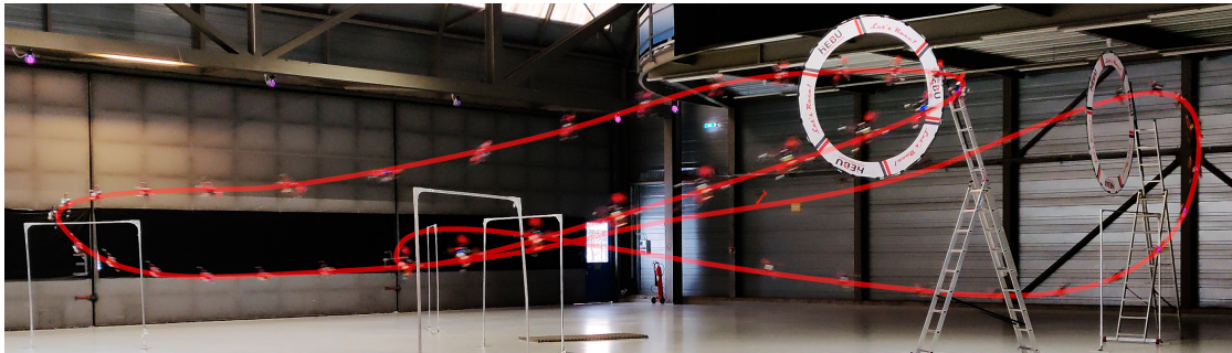
Figure A.1: A time-optimal trajectory. This time-optimal flight path was computed using the proposed complementary progress constraints (CPC) and executed in a motion capture system, outperforming the best human expert.
