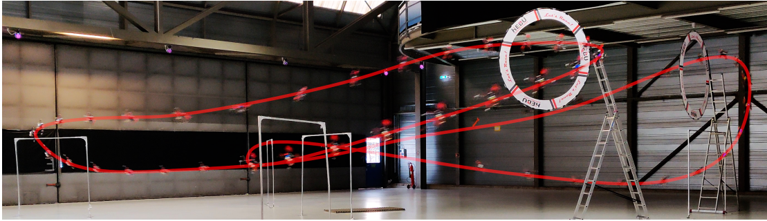
Figure 2.1: This time-optimal flight path was computed using the proposed complementary progress constraints (CPC) and outperforms expert human pilots.
