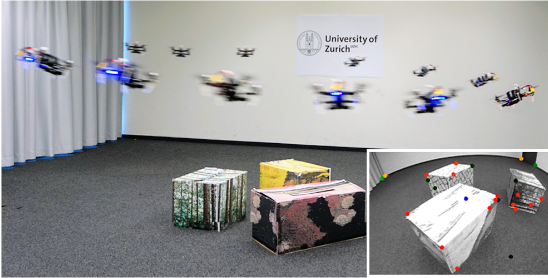
Figure G.1: An example application of our PAMPC, where a quadrotor is asked to fly at 3 \text{ m s}^{-1} around a region of interest while keeping it visible in the field of view of its camera.
