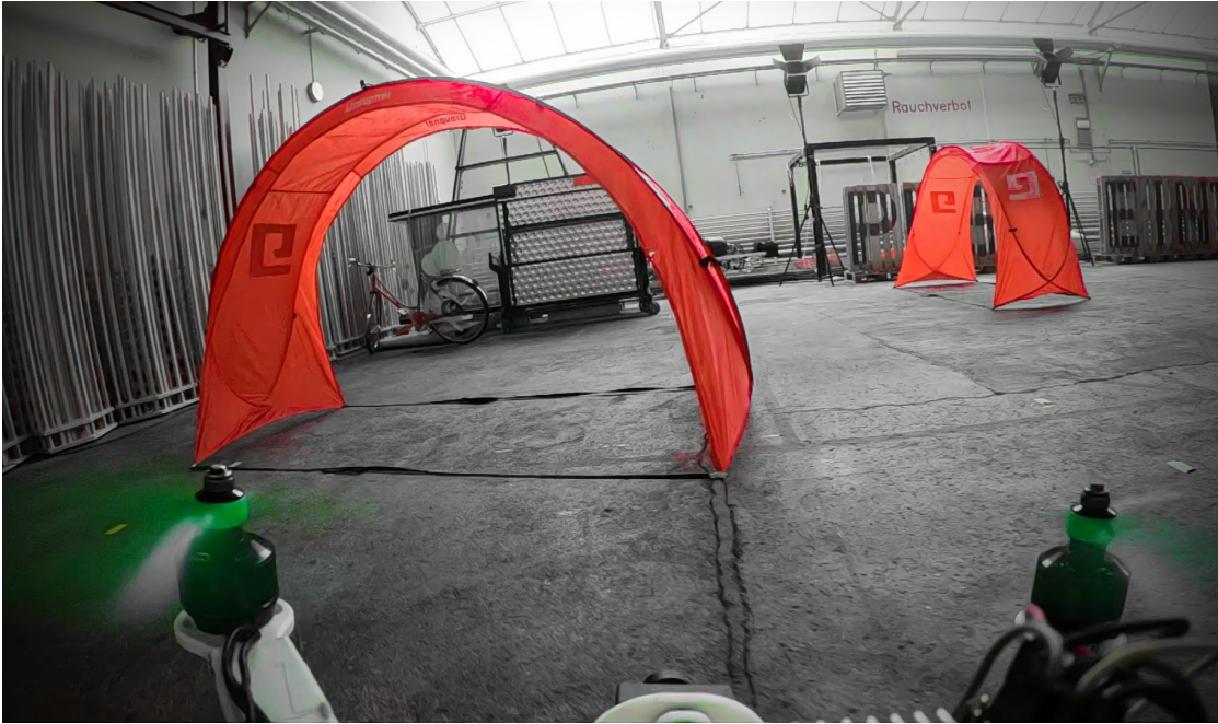
Figure F.1: A quadrotor flies through an indoor track. Our approach uses optimal filtering to incorporate estimates from a deep perception system. It can race a new track after a single demonstration.
