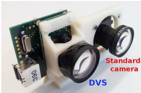
Fig. 7: An event camera (DVS) and a standard camera mounted on a rig. The standard camera was only used for comparison.
