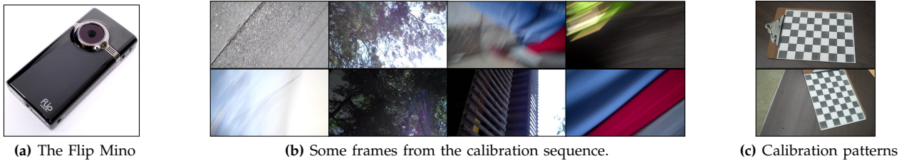
Figure 3: The FLIP camera is a consumer-level portable video recorder. The data for calibration is taken while walking in the Caltech campus, with the camera in hand, and "randomly" waving the arm, elbow, and wrist.
