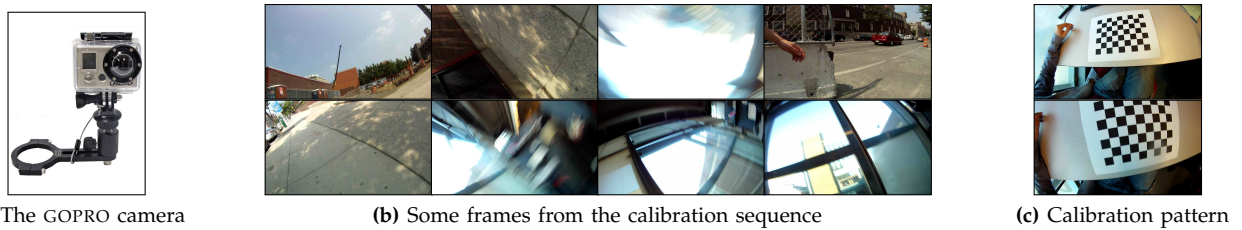
Figure 4: The GOPRO camera is a rugged consumer camera for outdoors use. It uses a fish-eye lens with 170° field of view.
