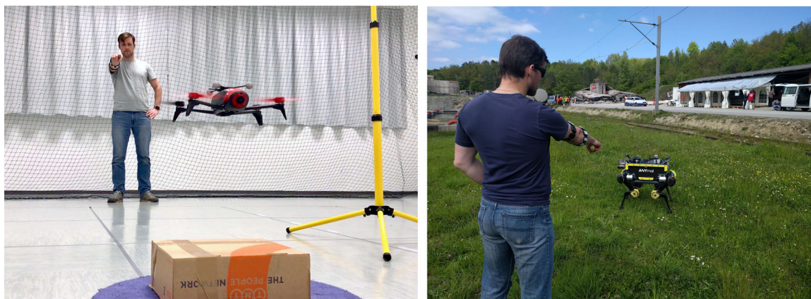
FIGURE 10 Human–robot interface from (Gromov et al., 2018, 2014), in which the operator uses pointing gestures, estimated from sensors worn in armbands, to provide navigation commands to both flying and legged robots [Color figure can be viewed at wileyonlinelibrary.com ]
