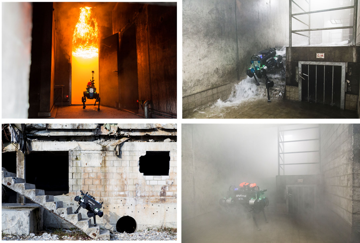
FIGURE 2 Modular quadrupedal robot ANYmal being deployed in challenging disaster environments (Hutter et al., 2017), highlighting its ability to navigate over rough terrain and in degraded sensing conditions, and demonstrating its resistance to fire and water [Color figure can be viewed at wileyonlinelibrary.com ]
