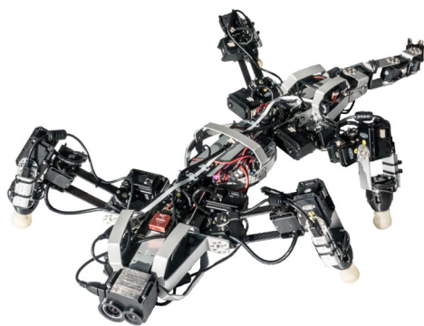
FIGURE 7 Amphibious robot Krock2, which uses a sprawling posture for crawling locomotion on land, is able to swim in water, and can maneuver through tight spaces using coordinated limb and spine actuation (Horvat et al., 2015, 2017b) [Color figure can be viewed at wileyonlinelibrary.com ]
