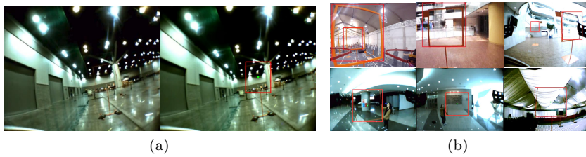
Fig. 6 Gate detection by KAIST (a) A racing gate of the ADR 2017 arena (left) and gate detection result using ADRNet (right) (b) Gate detection results on various backgrounds
