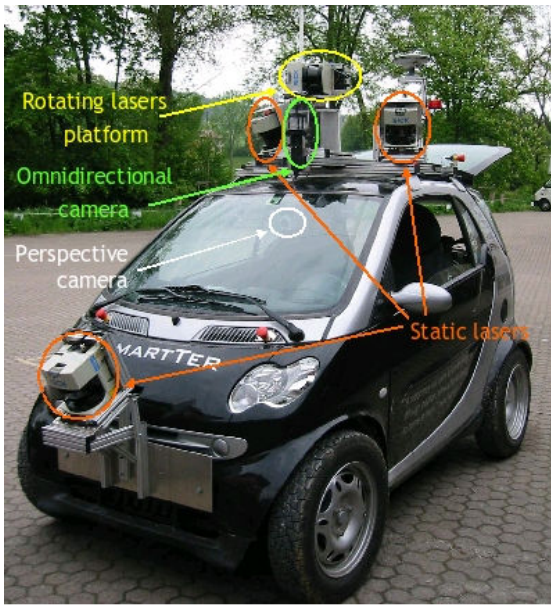
Fig. 1. The autonomous robot SmartTer developed at the Autonomous Systems Lab at the ETH Zurich. For the ego-motion estimation presented in this paper, we use the omnidirectional camera mounted on the roof, while the front laser, the perspective camera, and the rotating 3D scanner are used for detection and tracking of pedestrians and cars. The other static lasers are for collision avoidance, which is not covered in this paper.
