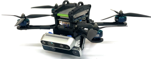
Fig. 8: Quadrotor used in real-world experiments.
