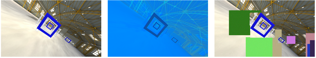
Fig. 3: Data augmentations used for training. Left: none. Middle: random convolution. Right: random cutout-color.
