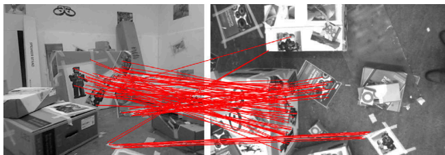
Fig. 3: Image feature matching results of the indoor scene using ASIFT [6]. Matches were found on planar textured surfaces. No matches were found in the outdoor scene depicted on the left of Figure 2.
