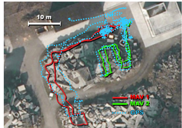
Fig. 16: Trajectories of the two MAVs in the outdoor experiment overlaid with the GPS measurements.
