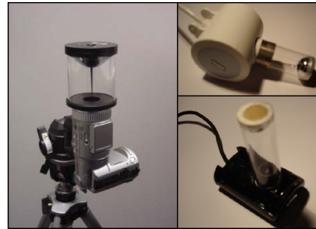
Fig. 1. Left: hyperbolic mirror placed on a video camera. Top right: Philips SPC 300. Bottom right: Philips ToUCam Fun.
