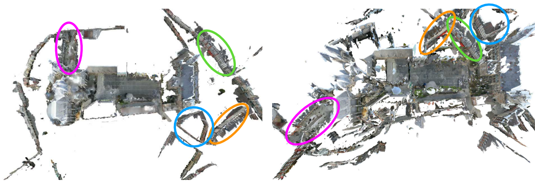
Fig. 2: Multi-View Stereo reconstructions obtained from SfM models of the Aachen dataset using SIFT (left) and D2-Net (right) features (top-down view). D2-Net features are more robust to changes in conditions, e.g., day-night and seasonal changes, than classic SIFT features, but also produce more false positive matches. This leads to connecting unrelated scene parts during the SfM process and ultimately in an incorrect 3D model. In contrast, SIFT correctly reconstructs the scene. Some wrong placements are illustrated through colored ellipses.
