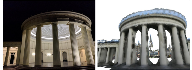
(b) Failure mode 2: scene with little texture.
