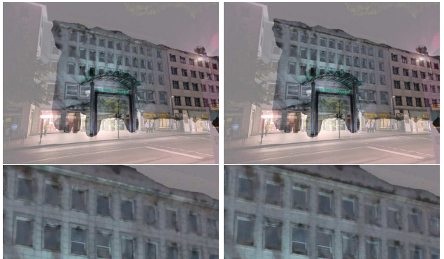
(c) Example where the SIFT pose (left) is more accurate than our method (right), as can be seen from the windows and the edge of the roof in the cutouts.
