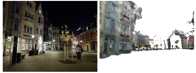
(a) Failure mode 1: low quality mesh.
