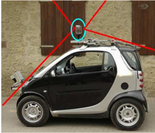
Fig. 1. Vehicle used in our experiments equipped with the omnidirectional camera (in the circle). The vertical FOV is indicated by the lines.
