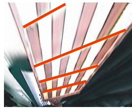
Figure 7. The sample image of Fig. 6 after rectification. Now the edges (highlighted) appear straight.
