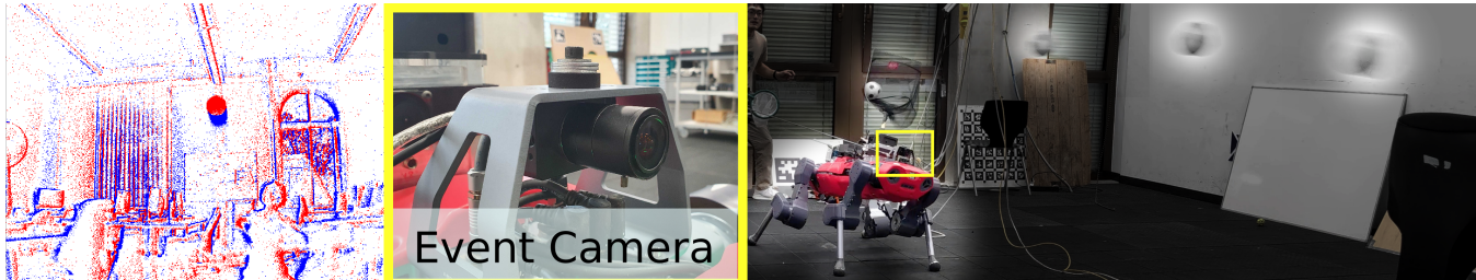
Fig. 1: Event-based agile object catching with a quadrupedal robot, using only onboard perception and control. By using the low latency of events, our robot is able to catch objects at speeds up to 15 m/s with a 83% success rate.
