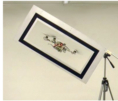
Fig. 5: Our quadrotor during a traverse.
