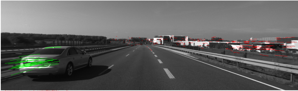
Fig. 2. Forward-Backward: car-mounted camera is moving forward passing another car which is also moving forward (moving backward with respect to the camera). Different colors represent the segmented trajectories.
