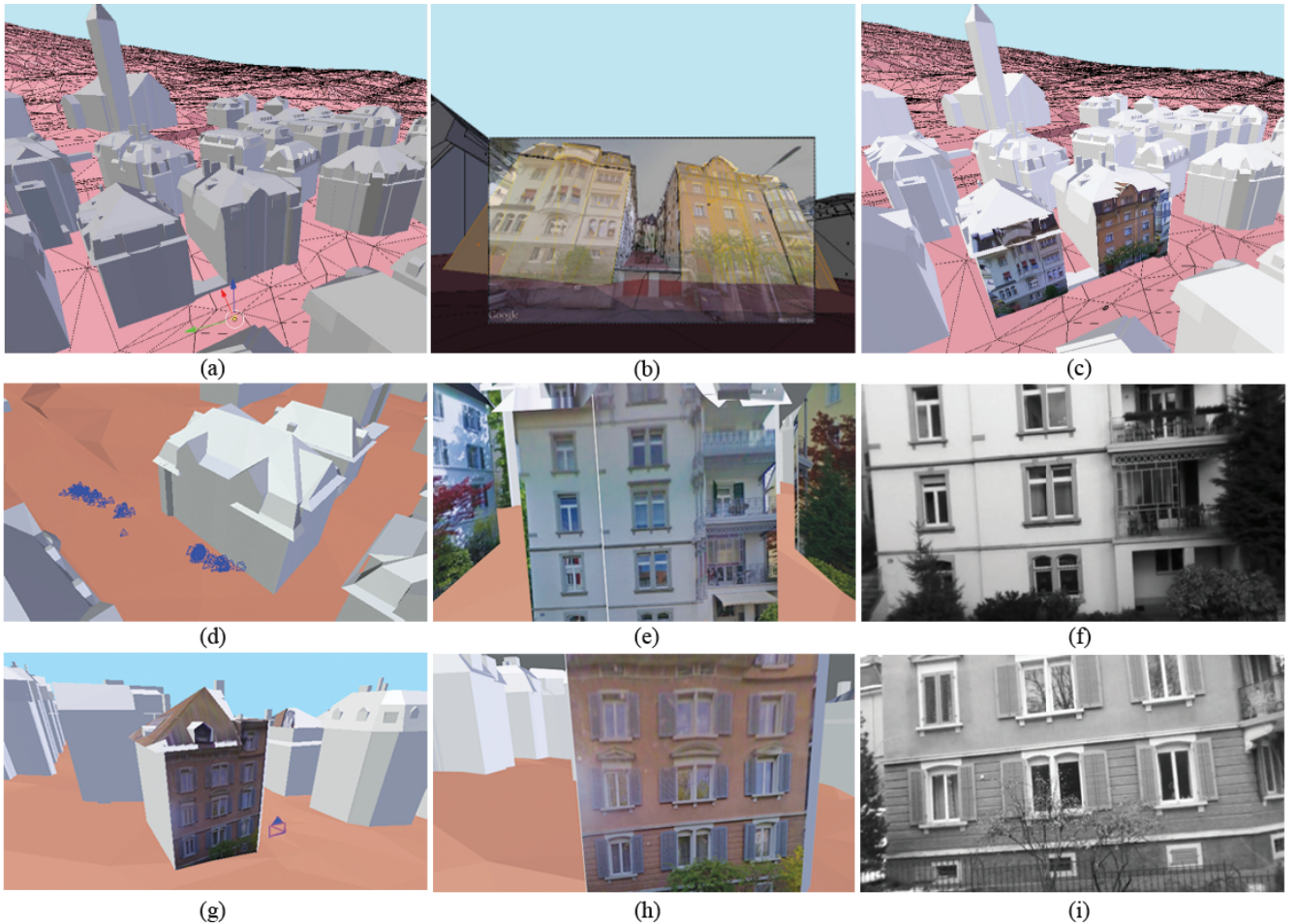
Fig. 5: (a) perspective view of the cadastral 3D city model; (b) the ground-level Street View image overlaid on the model; (c) the back-projected texture onto the cadastral 3D city model; (d) estimated MAV camera positions matched with one Street View image; (e) the synthesized view from one estimated camera position corresponding to actual MAV image (f); (g)-(i) show another example from our dataset, where (g) is an aerial view of the estimated camera position (h), which is marked with the blue camera in front of the textured 3D model, (h) is the synthesized view from the estimated camera position corresponding to actual MAV image (i).
