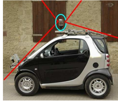
Fig. 6. The vehicle used in our experiments equipped with the omnidirectional camera (in the circle). The vertical field of view is indicated by the lines.
