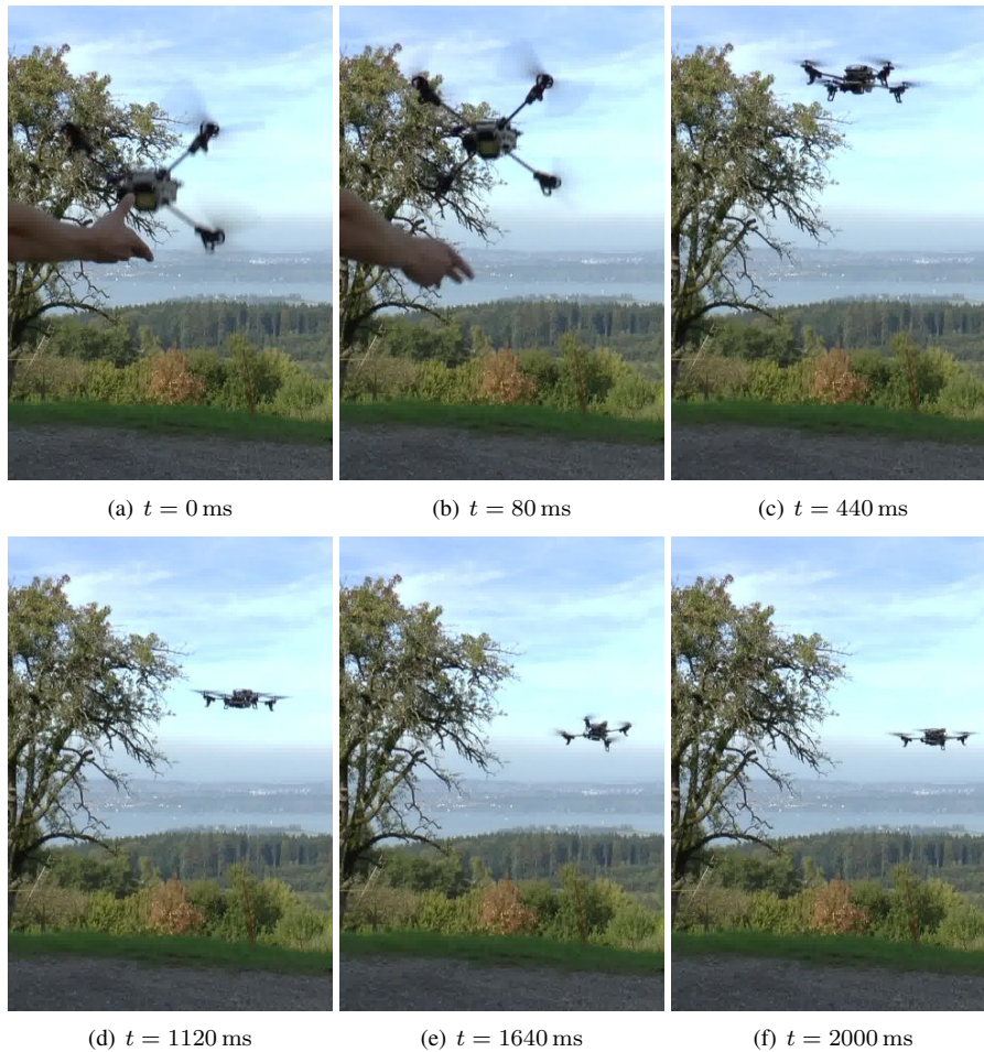
Figure 6.4 Autonomous recovery after throwing the quadrotor by hand: (a) the quadrotor detects free fall and (b) starts to control its attitude to be horizontal. Once it is horizontal, (c) it first controls its vertical velocity and then, (d) its vertical position. The quadrotor uses its horizontal motion to initialize its visual-inertial state estimation and uses it (e) to first break its horizontal velocity and then (f) lock to the current position. Image courtesy of (Faessler et al. 2015a).
