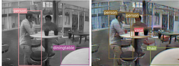
Figure 8: Object detection (YOLO [58]) on reconstructed images using E2VID. Color (right) tends to improve detection performance.
