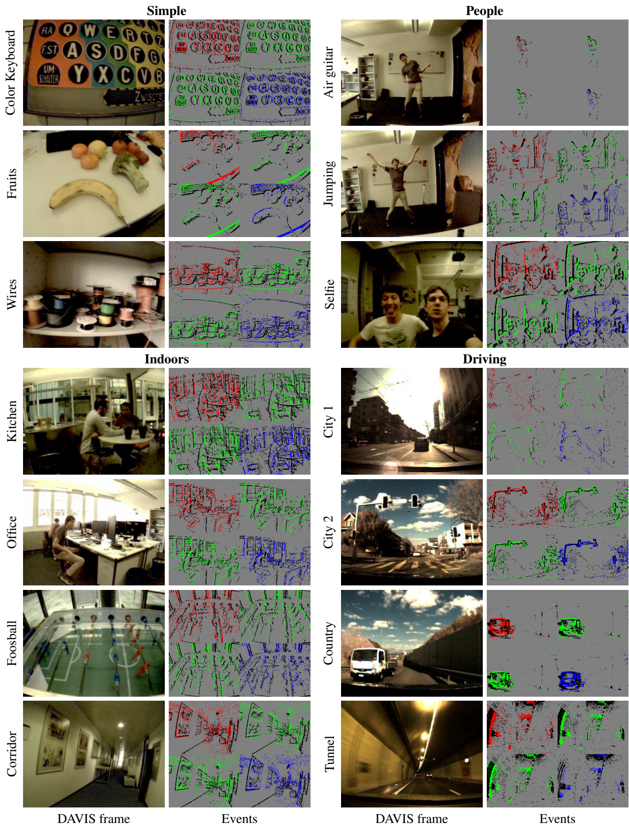
Figure 4: Impressions of the scenes from our dataset. Left column: color DAVIS frame; right column: color events.
